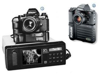
Nikon bodies, Kodak sensors, 1992 First DSLR 1.5 Mpix resolution; Tethered External Hard Disk Cost: up to \$20,000 Sold < 1000 units
