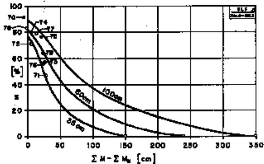
Figure 6 Nomograph of modified depletion curves for the elevation zone 2100-2600 m a.s.l., 24.5 km<sup>2</sup>, of the Dischma basin in the Swiss Alps. The curves are labelled with the average areal water equivalent of snow on the starting date 1 May. the position of points for the respective years indicate different snow reserves on 1 May.
