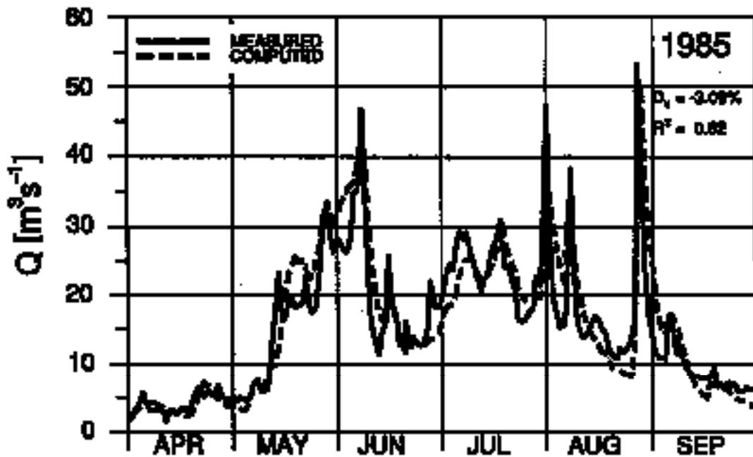
Figure 4 Computed and measured discharge from the catchment area of the hydroelectric station Tavanasa.  $D_v$  = difference of the total runoff volume,  $R^2$  = coefficient of determination.
