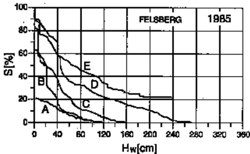
Figure 5 Modified depletion curves of snow coverage for the elevation zones A, B, C, D, E of the Felsberg basin, starting date 1 April 1985.
