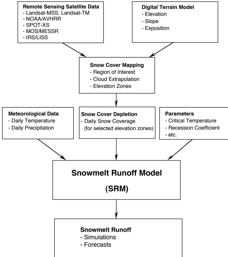
Figure 3 Flow chart for Snowmelt Runoff Modelling
