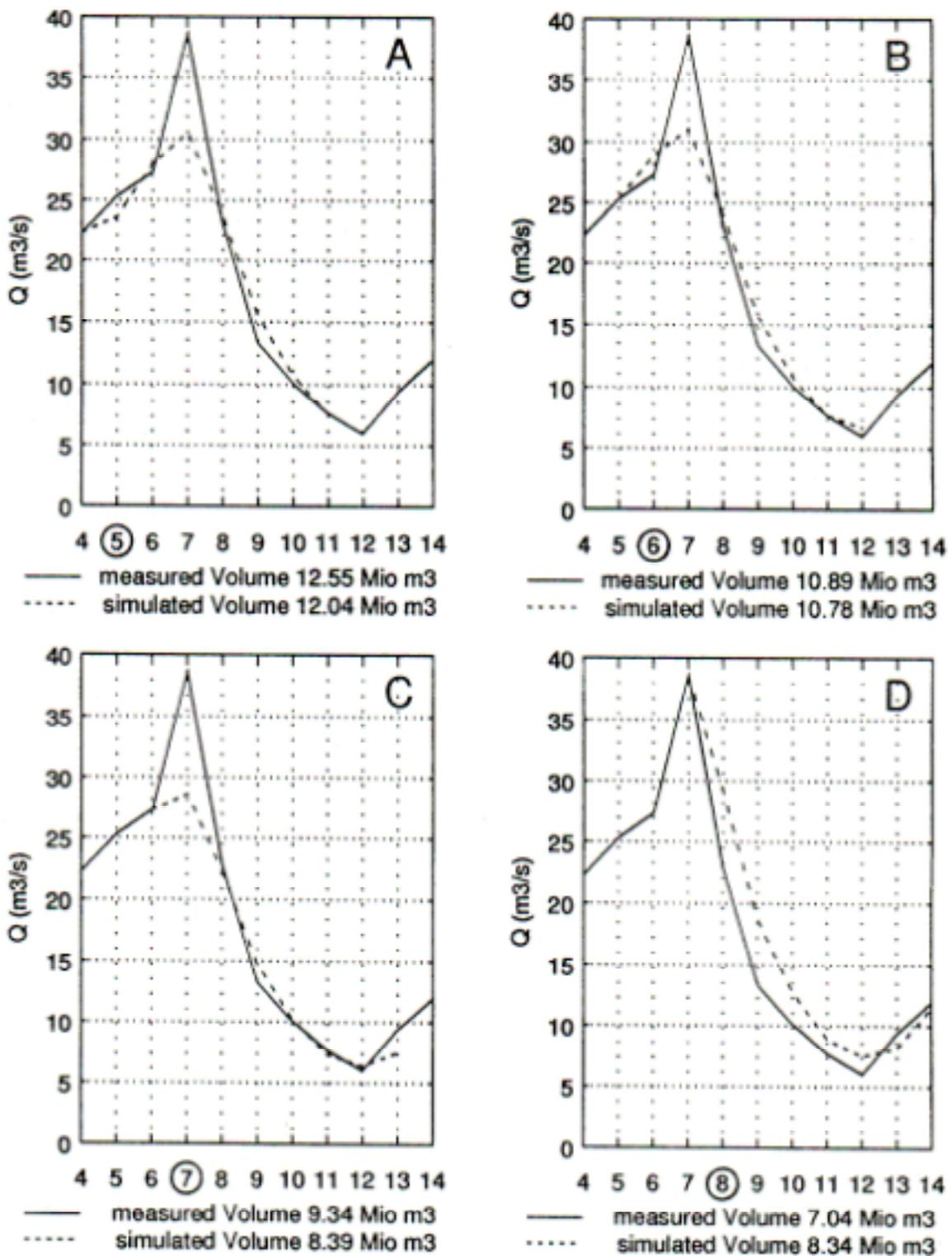
Figure 7 Simulated short term forecasts for the hydroelectric station Tavanasa.
