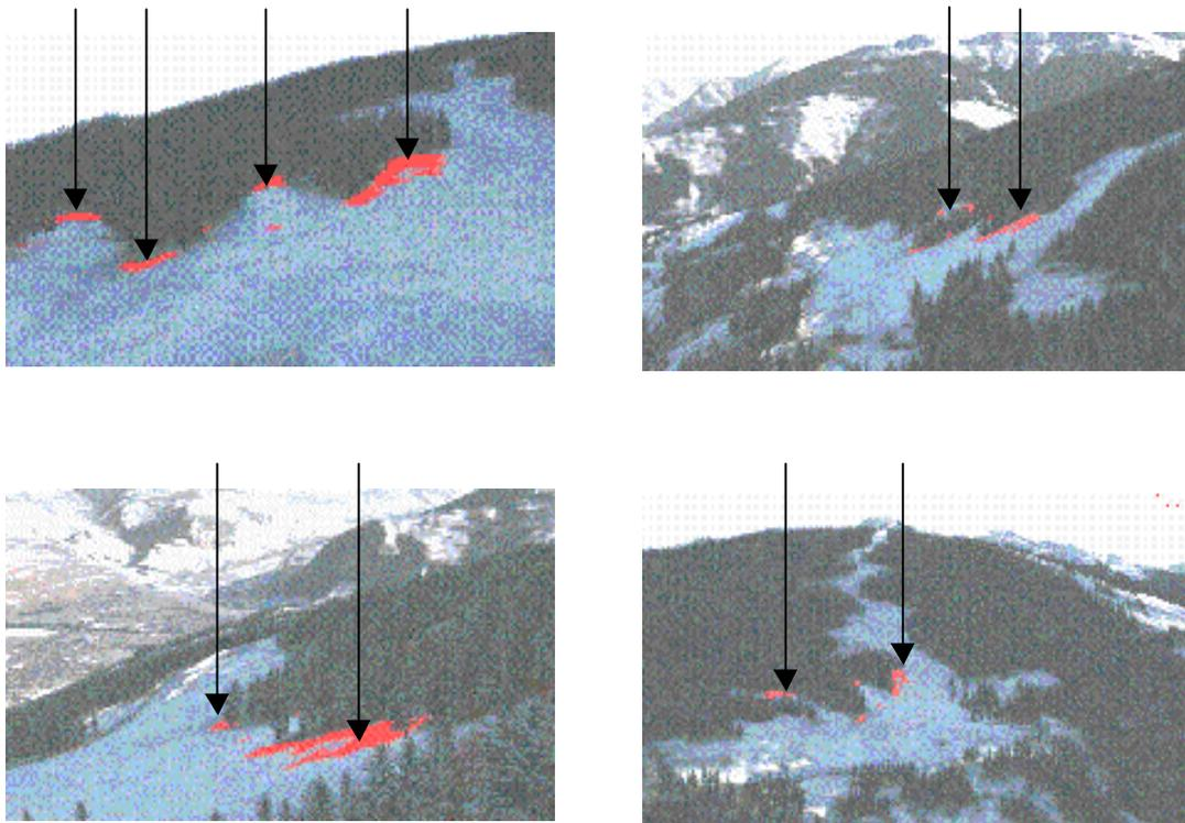
Fig. 9 Virtual pictures of the test site Veysonnaz. The arrows point to the grey shaded areas, which have to be cut for the free style slope. The pictures are the result of the overlay of aerial photographs over the digital elevation model in the foreground and of satellite data in the background.
