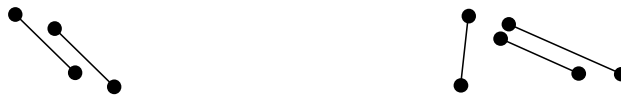
Fig. 1. Dots represent pixels. Pixels connected by lines represent cliques. Left: cliques of the same type, right: cliques of different types.
