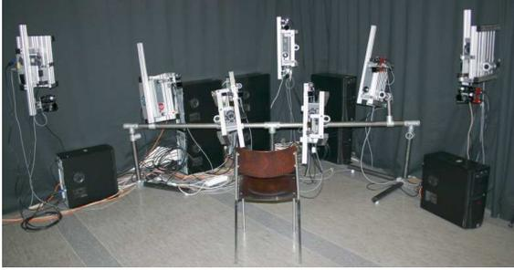
Figure 1. 3D-scanning setup for human face reconstruction: several cameras and projectors are positioned around the object of interest in a distance of approx. 1.5m.
