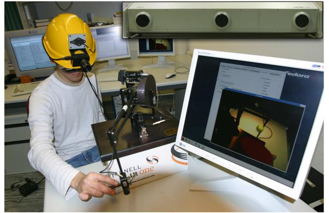
Figure 1: View depicting all components of AR system: head-mounted camera, marker, haptic device and optical tracking system (in the small window)
