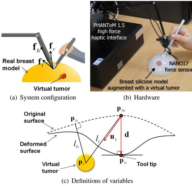
Figure 1: System configuration and variables definition.
