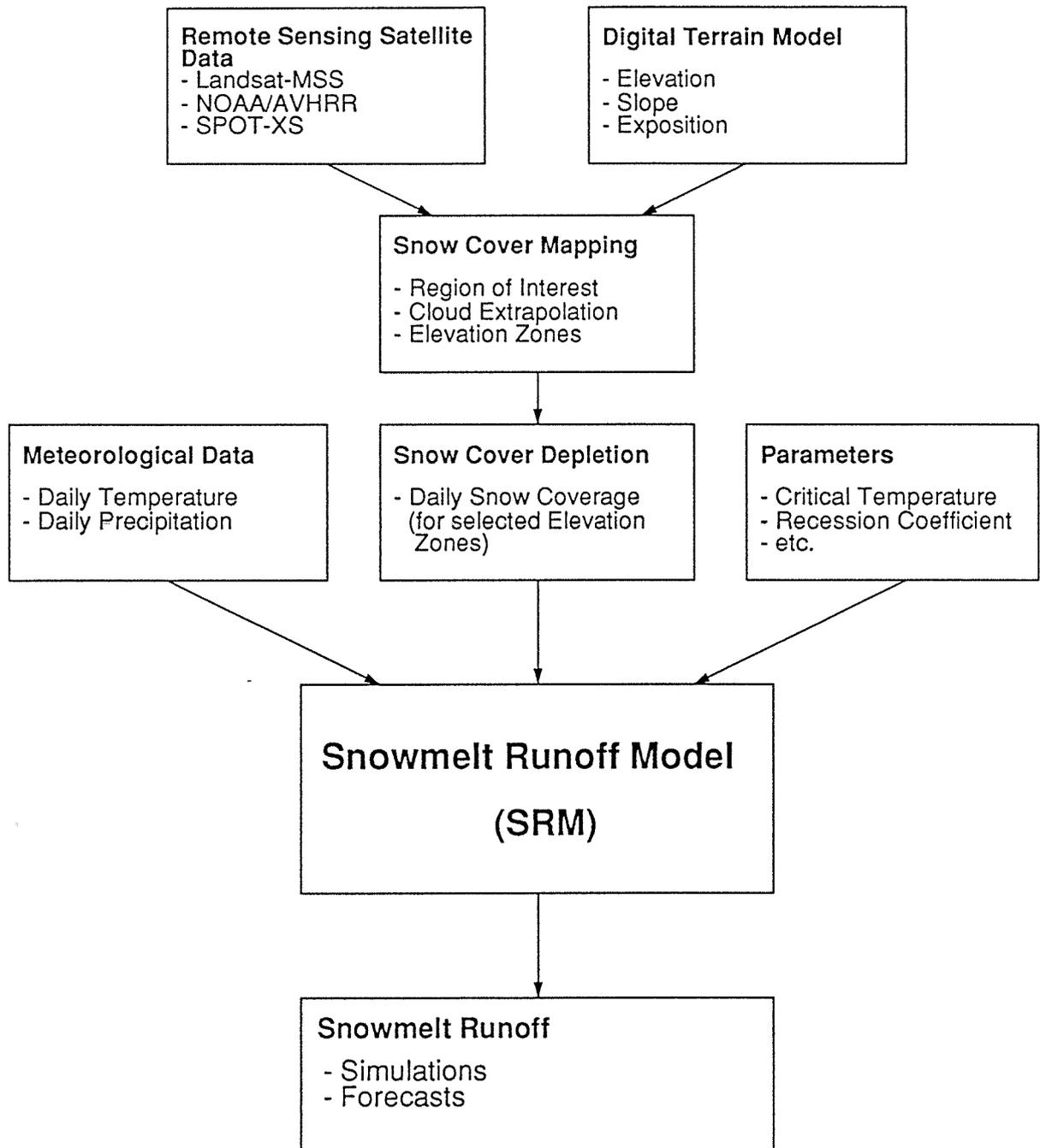
Fig. 2 Flowchart of the procedure of snowmelt runoff simulations based on remote sensing satellite data.
