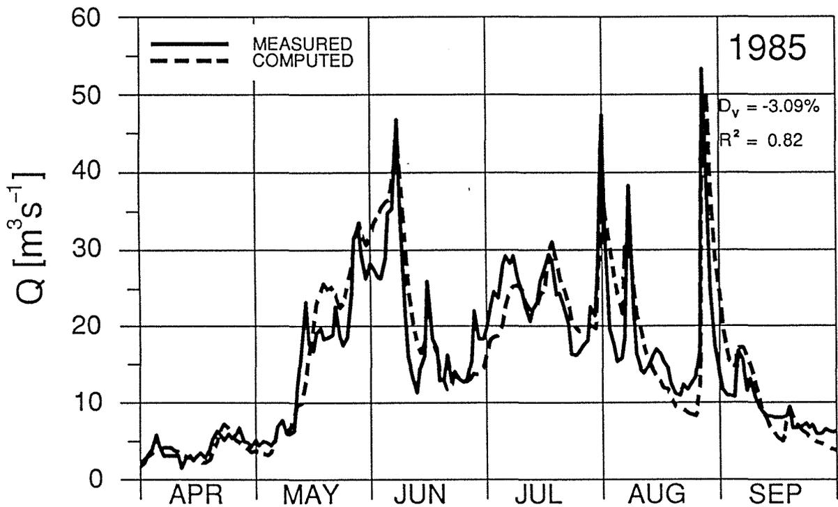
Fig. 5 Computed (---) and measured (—) discharge from the catchment area of the hydroelectric station Tavanasa.
