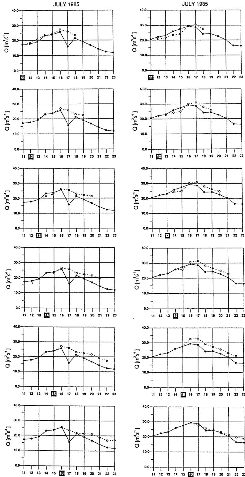
Fig. 6 Weekly forecasted (---) and measured (—) runoff for the power stations Sedrun (left) and Tavanasa (right). Starting day is marked reversed.
