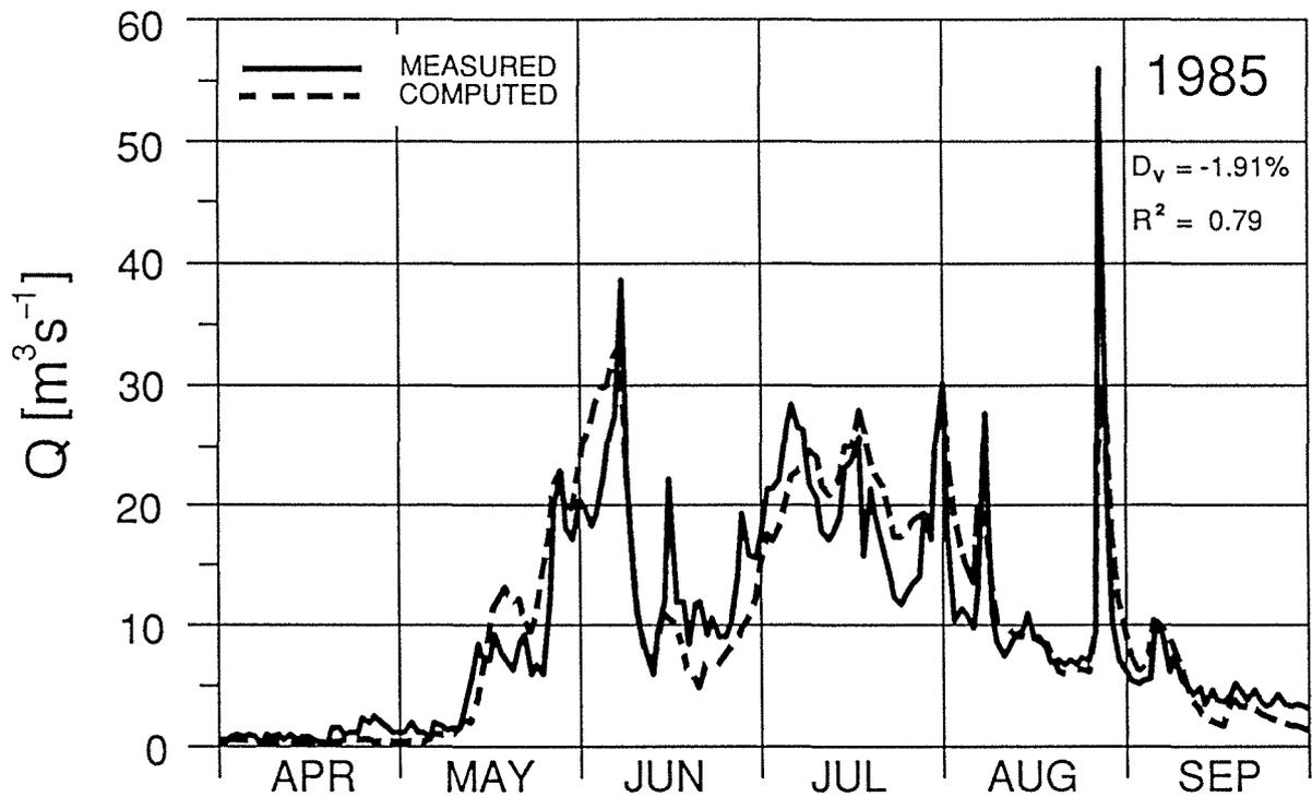
Fig. 4 Computed (---) and measured (—) discharge from the catchment area of the hydroelectric station Sedrun.
