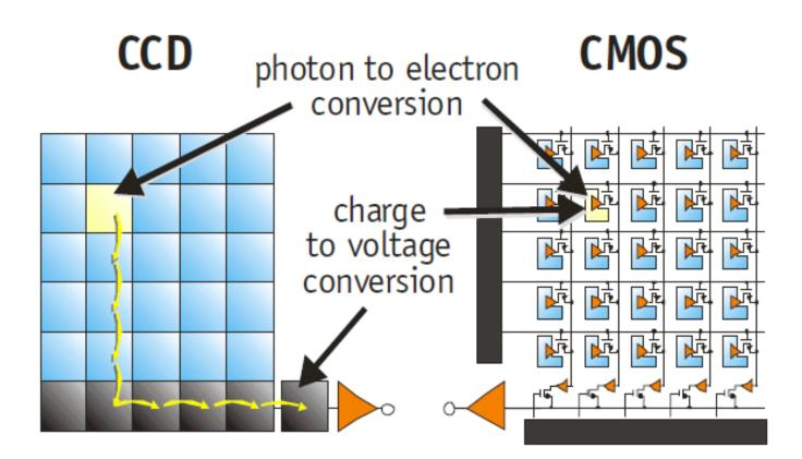
CCD = Charge-coupled device CMOS = Complementary Metal Oxide Semicond<sup>®</sup>uctor
