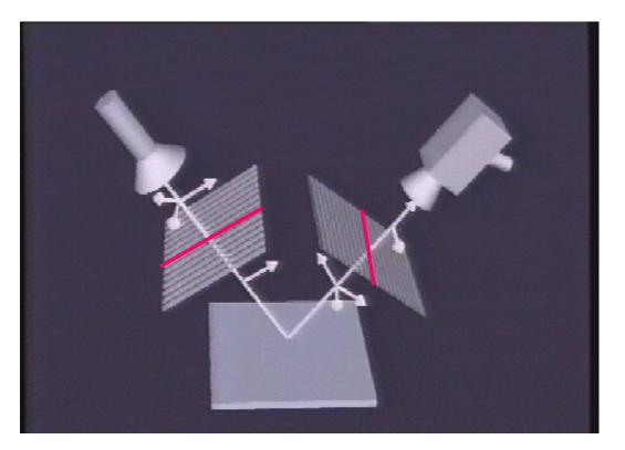
polarizer/analyzer crossed prevents the large dynamic range caused by glare
