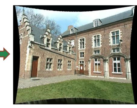
This aberration type can be corrected by software if the parameters (  $\kappa_1$  ,  $\kappa_2$  , ... ) are known <sup>45</sup>
