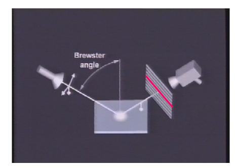
polarizer/analyzer aligned distinguished metals and dielectrics
