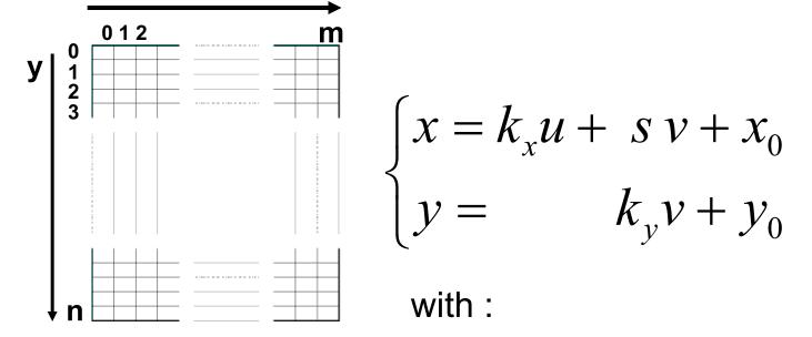
**NB3** : *kx*,*ky*,*s*,*x0* and *y0* are called *internal camera parameters*
