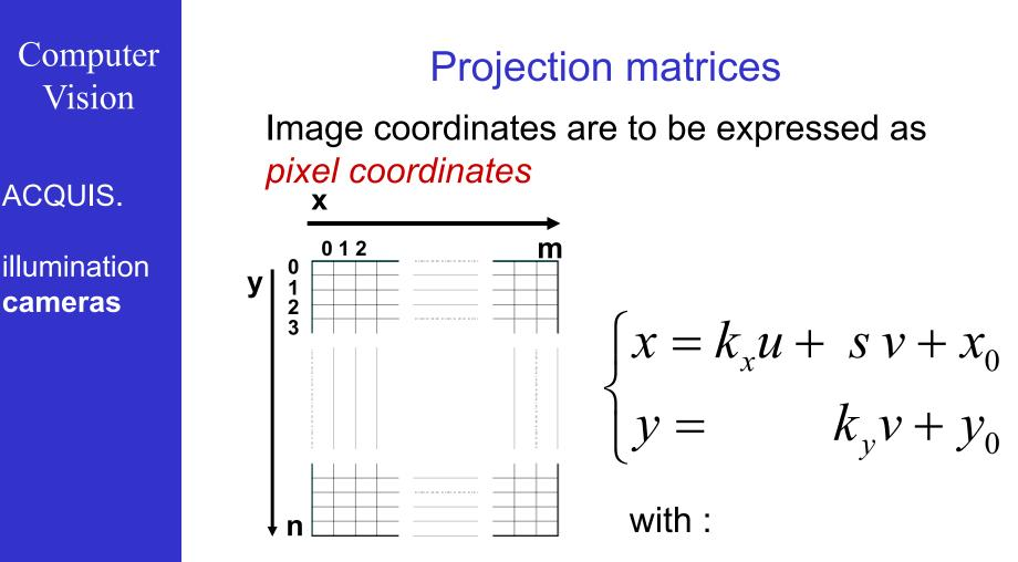
→ (x0, y0) the pixel coordinates of the principal point →  $k_x$  the number of pixels per unit length horizontally →  $k_y$  the number of pixels per unit length vertically → s indicates the skew ; typically s = 0
