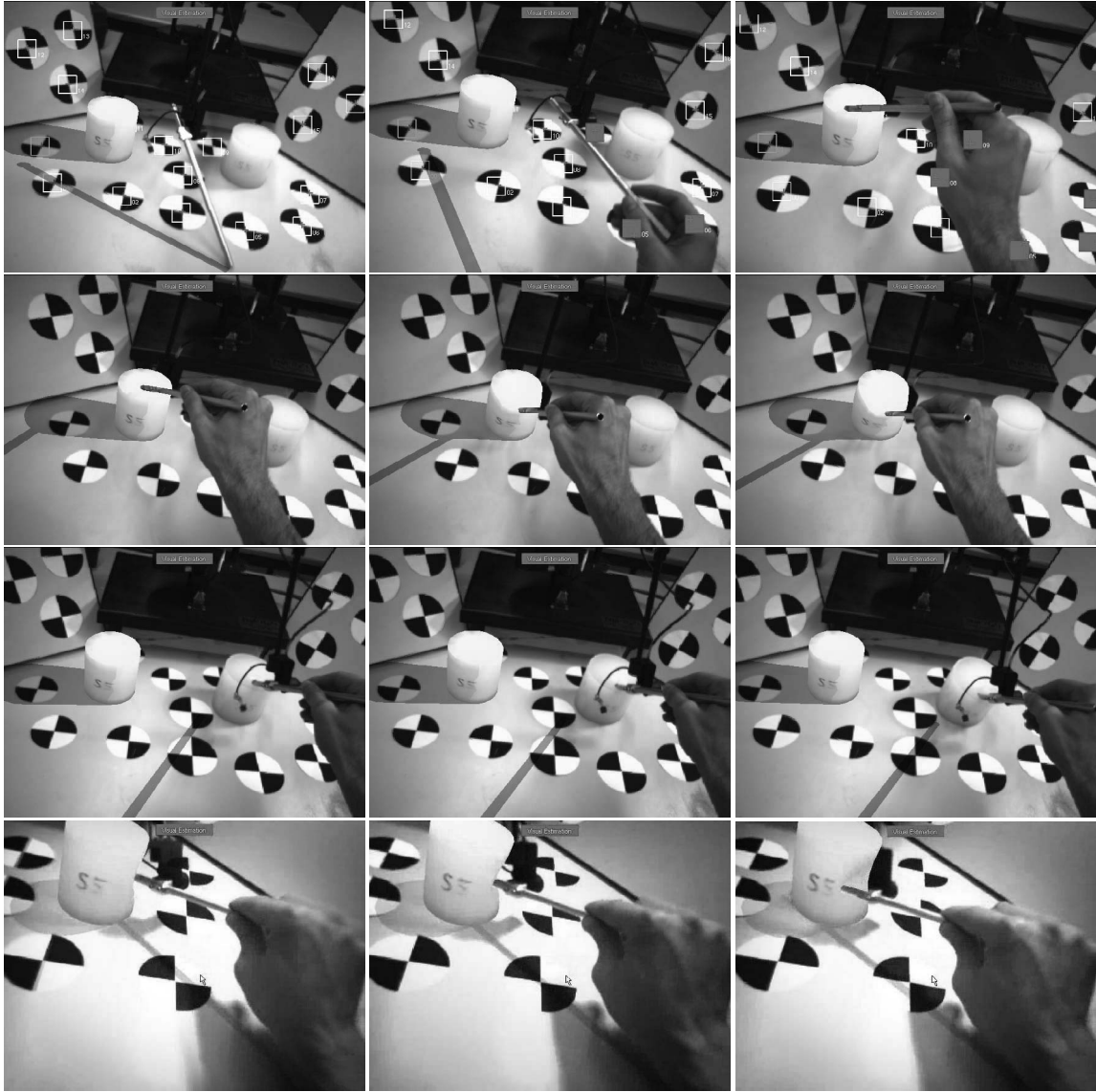
Figure 12: From the top, the first row shows the AR scene with detected landmarks. The second row illustrates the interaction between the haptic device and the deformable object. The third row depicts similar actions on the real object. The last row provides a close view of the deformations.
