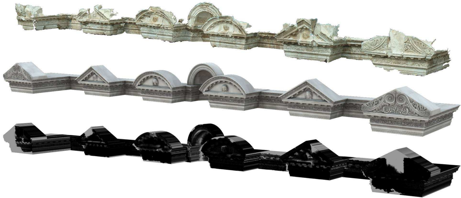
Figure 7: Comparison of captured 3D data (top) and the reconstructed model (middle). High intensities in the bottom figure correspond to large differences between these two and hence large uncertainties.
