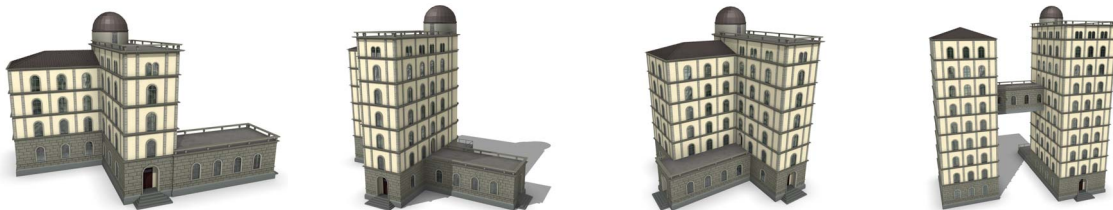
Figure 5. This figure shows the application of CGA shape , a novel shape grammar for the procedural modeling of computer graphics architecture. First, the grammar generates procedural variations of the building mass model using volumetric shapes and then proceeds to create facade detail consistent with the mass model. Context sensitive rules ensure that entities like windows or doors do not intersect with other walls, that doors give out on terraces or the street level, that terraces are bounded by railings, etc.
