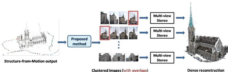
Figure 1: The overall scheme of a reconstruction using camera clustering.
